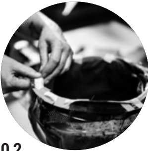
02 The material is placed into the mould by hand, layer by layer.
