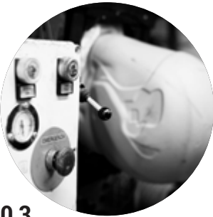
03 The shell is hardened under heat and pressure – around 180°C.
