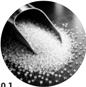
01 Polycarbonate granules are heated to approx. 300°C until liquefied.
