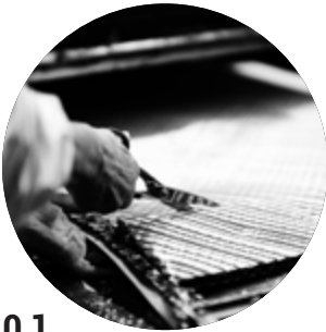
01 Fibre mats are cut to shape – including fiberglass, Kevlar and carbon.
