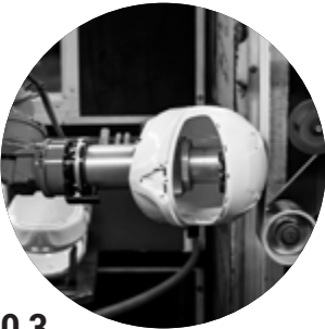
03 The shell cools, hardens and is precisely finished.
